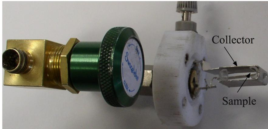
**FIGURE 14.** Photograph of the sample-collector assembly.
