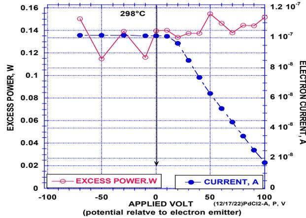
**FIGURE 16.** Electron current and the excess power at a temperature of  $298^{\circ}\text{C}$  when the voltage between the emitter and collector is changed. The potential is shown relative to the emitter.
