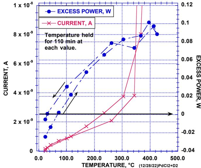
**FIGURE 15.** Excess power and emitted electron current are measured as a function of temperature when co-deposited Pd is heated in  $D_2$  gas. The electron emitter is held at 0 V relative to the collector. The arrows indicate the sequence of the measurements. The excess power was measured before the current was measured. The current was then measured when the temperature was increased and then decreased. The temperature is measured inside the cell but not in the sample.
