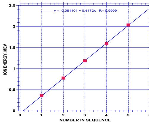
**FIGURE 11.** The relationship between the sequence in the spectrum and the ion energy when the first peak is given a value of 1.
