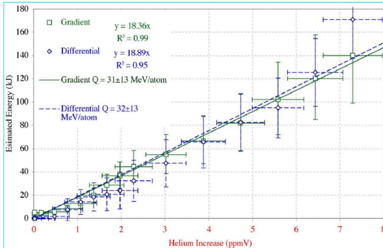
**FIGURE 8.** Energy and helium were made by a special batch of coconut charcoal to which 5% Pd was applied as fine particles and heated near 243°C in D<sub>2</sub> gas while energy and helium were measured as reported by McKubre et al.
