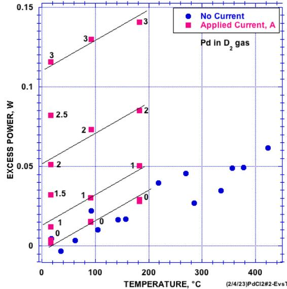
**FIGURE 6.** Effect of a steady DC passing through PdD at various temperatures in  $D_2$  gas. The amount of applied current is shown in units of ampere(A). The values for “no current” were obtained first followed by the values designated as “applied current”.
