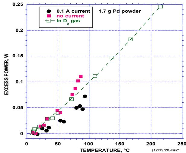
**FIGURE 2.** Excess power is a function of temperature when a sample of PdD is heated in the electrolytic cell or when it is heated in D<sub>2</sub> gas. Production of power at the higher temperatures continued even after the current to the sample is stopped in the electrolytic cell. No detectable power was found at the lowest temperature.
