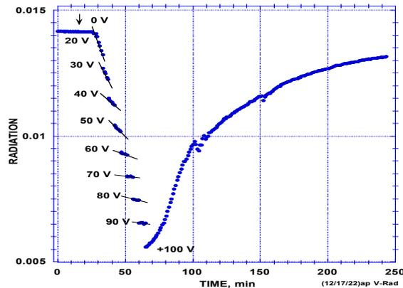
**FIGURE 17.** Effect of time on the voltage measured across a series resistor when the voltage across the cell is changed as shown in Fig. 16.
