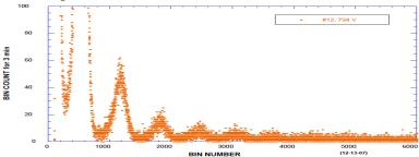
**FIGURE 10.** A typical spectrum is produced during gas discharge when either  $H_2$  or  $D_2$  is used. The bin number was calibrated using the energetic alpha emitted from  $Po^{210}$ .
