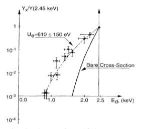
**FIGURE 18.** D+ bombardment of Ti with kinetic energy to produce the plotted rate of hot fusion relative to when a kinetic energy of 2.45 KeV [61] is applied. A calculated value for the screening potential  $(U_e)$  is shown. The bare cross-section is obtained when fusion occurs in plasma. The absolute fusion rate at this energy is near the detection limit, to which electron screening adds very little to the very small fusion rate.
