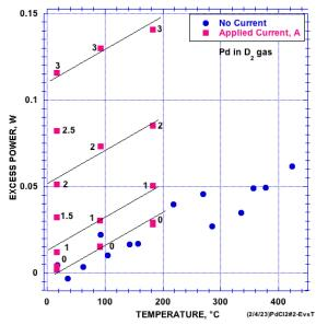
**FIGURE 6.** Effect of a steady DC passing through PdD at various temperatures in  $D_2$  gas. The amount of applied current is shown in units of ampere(A). The values for "no current" were obtained first followed by the values designated as "applied current".
