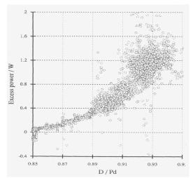
**FIGURE 4**. Effect of D/Pd ratio on power production when an active batch of Pd wire was reacted in an electrolytic cell near 20° C. McKubre et al. [25]
