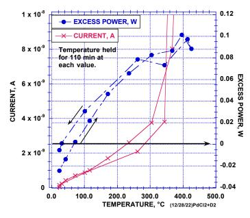
**FIGURE 15.** Excess power and emitted electron current are measured as a function of temperature when co-deposited Pd is heated in  $D_2$  gas. The electron emitter is held at 0 V relative to the collector. The arrows indicate the sequence of the measurements. The excess power was measured before the current was measured. The current was then measured when the temperature was increased and then decreased. The temperature is measured inside the cell but not in the sample.
