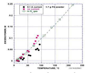
**FIGURE 2**. Excess power is a function of temperature when a sample of PdD is heated in the electrolytic cell or when it is heated in  $D_2$  gas. Production of power at the higher temperatures continued even after the current to the sample is stopped in the electrolytic cell. No detectable power was found at the lowest temperature.
