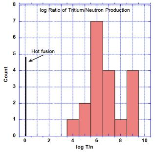
**FIGURE 9.** Histogram of published measurements of the log tritium/neutron ratio. The measured log T/n resulting from hot fusion is also plotted. The values are from Table 6, "The Science of Low Energy Nuclear Reaction".[5]
