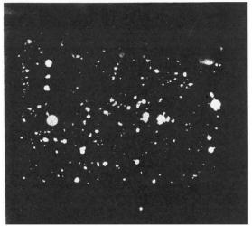
**FIGURE 13.** Spots are produced on photographic film by photons that passed through 0.5 mm of aluminum. A similar pattern is produced when 2 mm of Pb is used.
