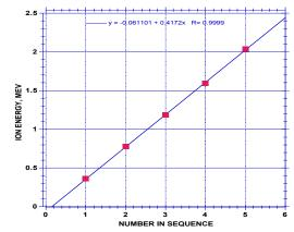
**FIGURE 11.** The relationship between the sequence in the spectrum and the ion energy when the first peak is given a value of 1.
