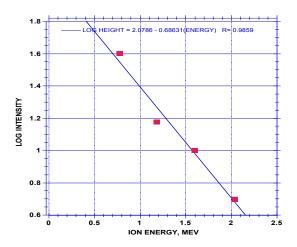
**FIGURE 12.** The relationship between log intensity and ion energy. The intensity is given as a relative value.
