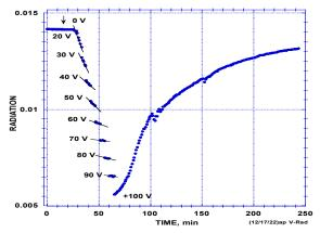
**FIGURE 17.** Effect of time on the voltage measured across a series resistor when the voltage across the cell is changed as shown in Fig. 16.
