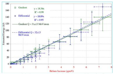
**FIGURE 8**. Energy and helium were made by a special batch of coconut charcoal to which 5% Pd was applied as fine particles and heated near  $243^{\circ}$ C in  $D_2$  gas while energy and helium were measured as reported by McKubre et al.
