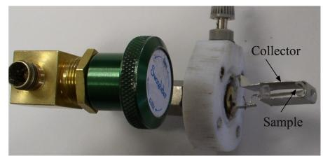
FIGURE 14. Photograph of the sample-collector assembly.
