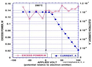
**FIGURE 16.** Electron current and the excess power at a temperature of 298° C when the voltage between the emitter and collector is changed. The potential is shown relative to the emitter.
