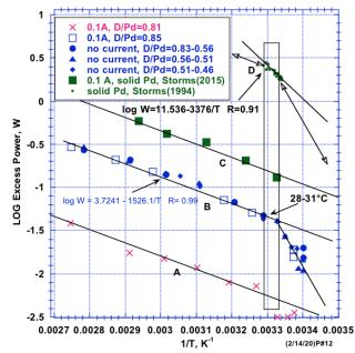
**FIGURE 3.** Comparison between the behaviors of different samples of solid and pressed powdered Pd when heated in an electrolytic cell. The designations A, B, C, and D apply to independent measurements. The lines drawn through each measurement are parallel, showing that each has the same activation energy.[19, 22]. The study labeled "D" fell in the transition temperature region between two different values for the activation energy. Storms(1994)[23]
