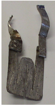
FIGURE 5. Sample of Pd coated with electrodeposited Pd and cut to allow the passage of a current through the metal. The cross-section through which the current passes is about 1 mm x 3 mm. The Pd weighs 2.5 g. (To be published)
